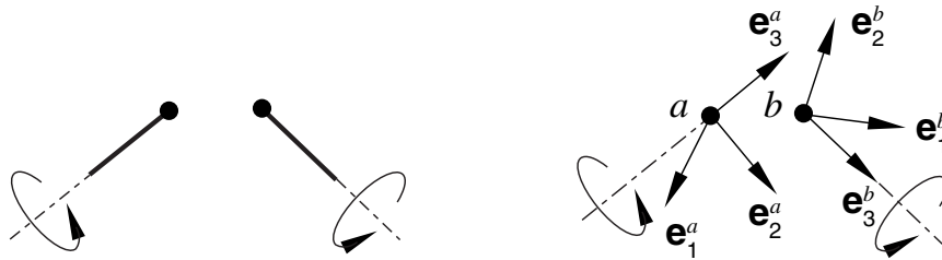
Figure 31.1.5-9 Connection type CONSTANT VELOCITY.
